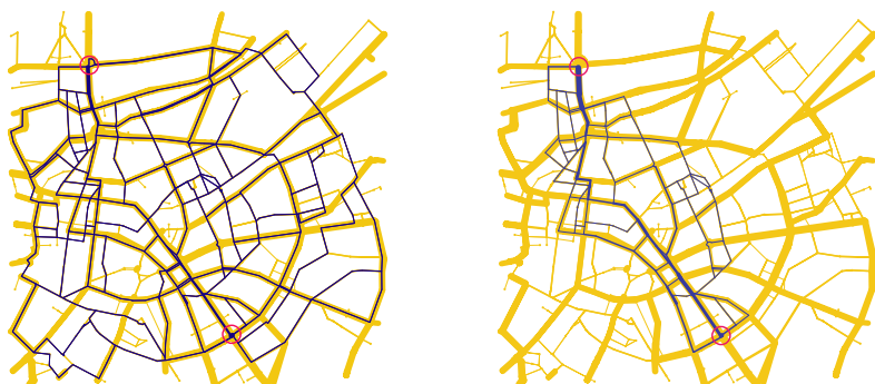
Fig. 5. System optimum with restrictions on path lengths: One commodity routed through the road network between the marked nodes. The left-hand side image displays the system optimum in which flow is distributed over the whole network in order to avoid high arc flows that would incur high arc transit times. In the right-hand side image the same amount of flow gets routed, but this time with a restriction on the geographical path lengths. Line thickness denotes arc capacity (yellow) and arc usage (blue).
